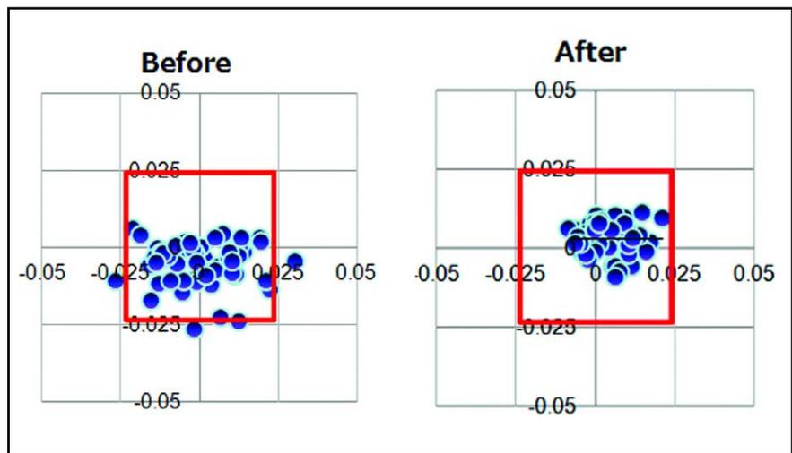
**The result of feedback from Saki's 3D AOI system to Panasonic's placement equipment during testing (unit = mm).**
